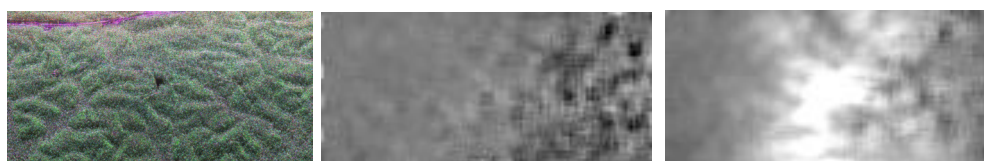
Figure 4: Example of two disparity maps (range (middle image) and azimuth (right image)) obtained on UHF band data from the SETHI sensor of ONERA on the Paracou dataset (left image) [15]. The two disparity images are scaled from -0.5 pixels (black) to +0.5 pixels
